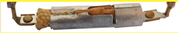
Slow-breaking heating blanket temperature limiter, used in conjunction with an English power control system made by GEC (General Electric Company). It is covered with a waterproof PVC sleeve, welded to the wires. Around 1970 (Ultimheat Collection)
