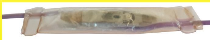
Slow-breaking heating blanket temperature limiter, used in conjunction with an English power control system made by GEC (General Electric Company). It is covered with a waterproof PVC sleeve, welded to the wires. Around 1970 (Ultimheat Collection)
