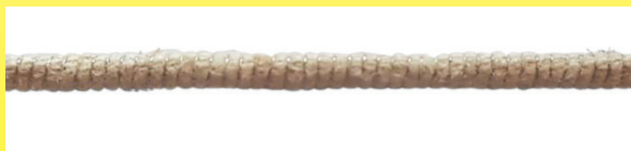
1960 ca. Calor heating cord, diameter 1.7mm, single nickel chromium heating wire, diameter 0.08mm, on a slightly twisted cotton core to prevent buckling (Ultimheat collection)
